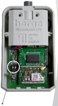
Removing the rear panel gives the user access to switches for setting the latency of the system and sleep timeout of the connected transmitters
